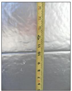
**Photo No. 7** Post-test, Witness Panel Impact
