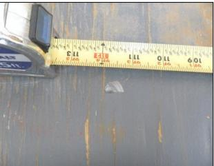
**Photo No. 6** Post-test, Witness Panel Impact
