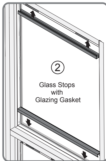
Install horizontal glass stops. Note: Horizontals run through.
