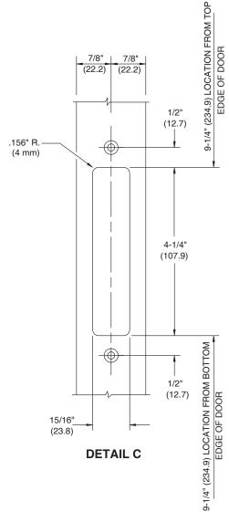
NOTE: Topflush bolt cut-out location for door opening height of 84" (213.4 cm) or less should be 9-1/4" (234.9) from top edge of door. See DETAIL A
