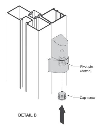
To remove existing doors with intermediate pivots, Remove cap screw and lower pivot pin to clear.
