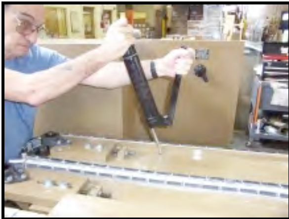
Figure 20 Conveyor Idler Sprocket Lubrication
