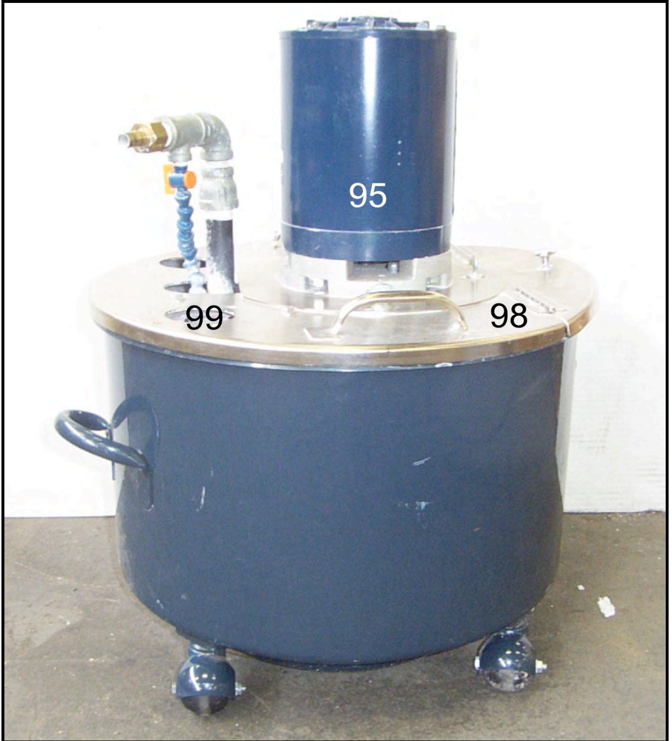
Picture 18 Cerium Tank, Pump and Screen Filter
