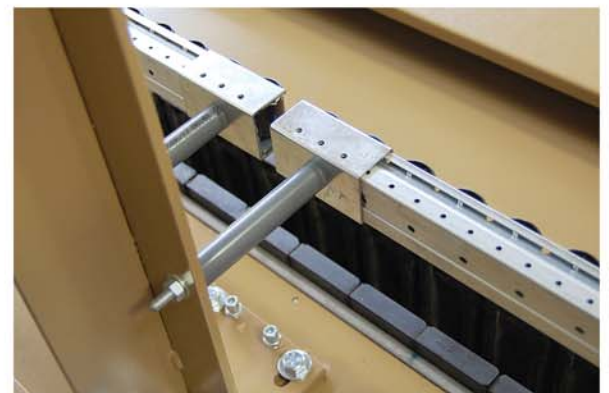
Two upper rails attached to the center upright
