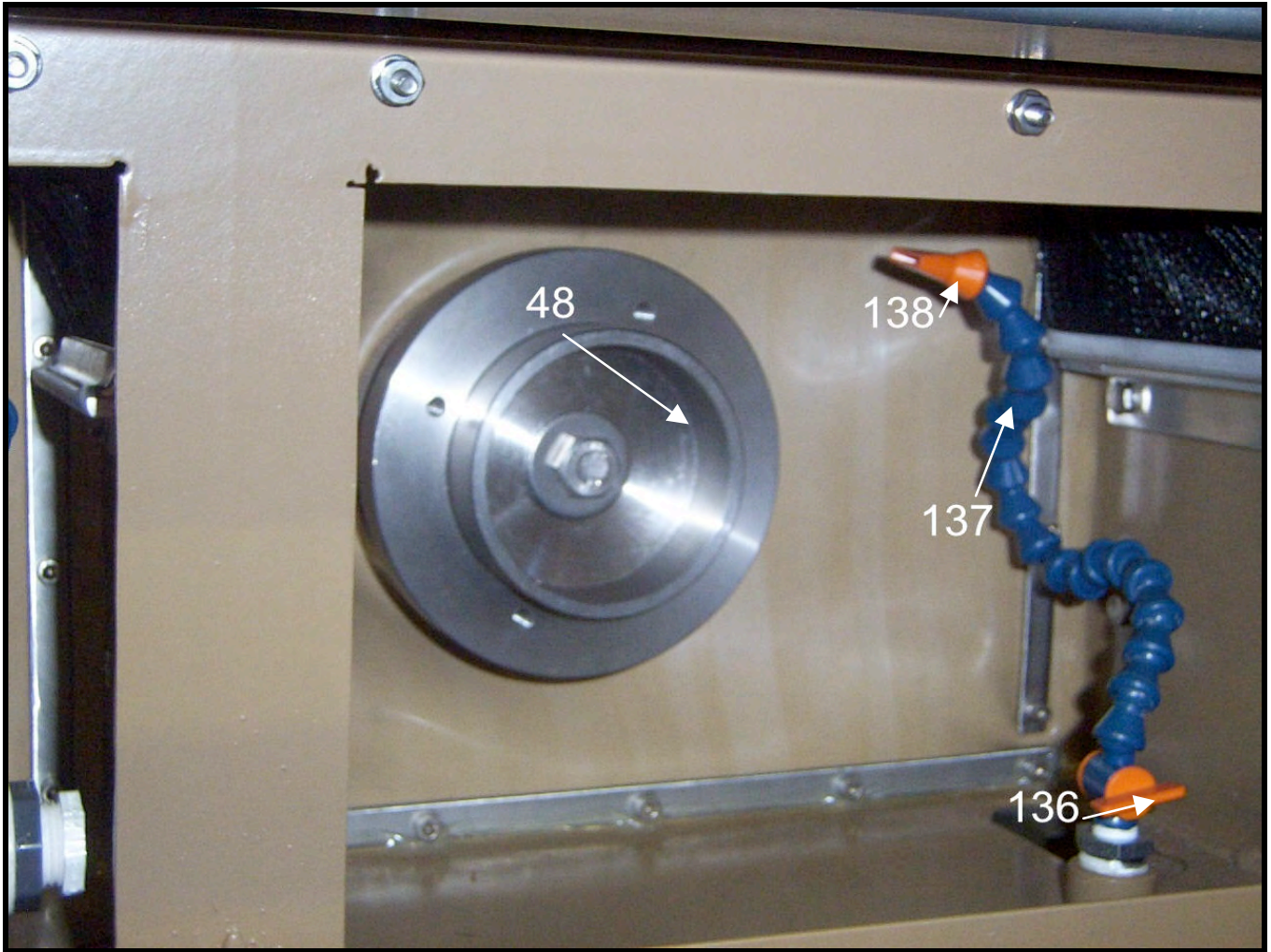
Picture 11 Cerium Polishing Section Hub and Cerium Lines
