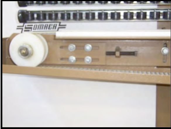
Figure 13 Ingoing Conveyor Belt Pulley
