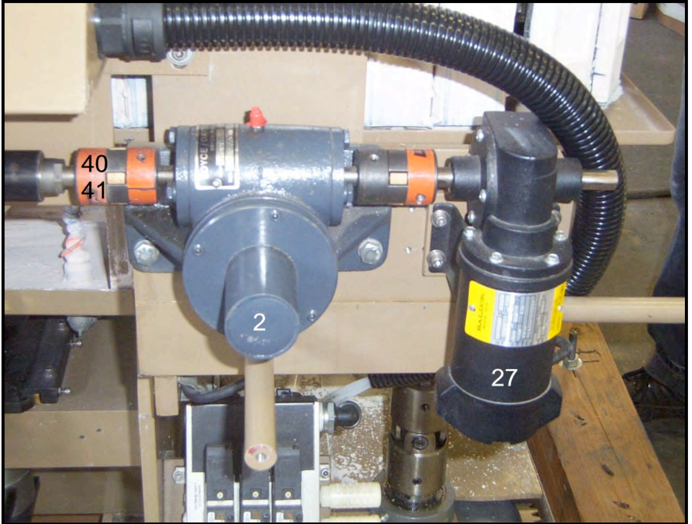
Picture 4 Right Side Front Tube Adjustment Jacks, Drive Motor and Couplings
