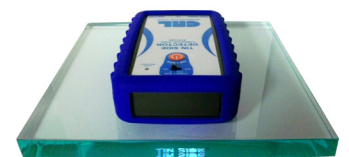
Figure 5: Stenciled image on tin side of glass
