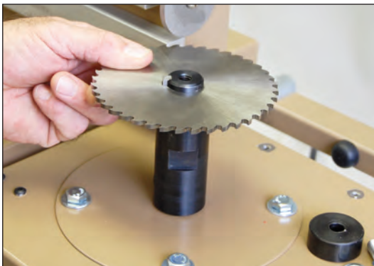
3. Be sure to retain the spindle key when changing the blade
