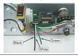
Step 5. Use the three tap connectors (provided) to splice power supply leads into units 120VAC power. Splice Black to Black; White to White; and Green to Green.
