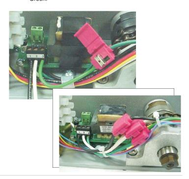
**Step 6.** Mount RF receiver to unit as shown using Velcro strip provided.
