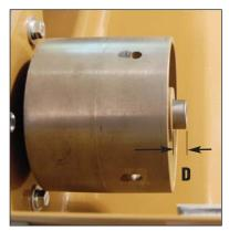
**Photo 4.** Measure Pulley to Shaft End distance "D" before removing Motor Pulley.
