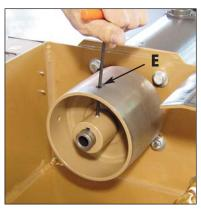
**Photo 5.** Loosen two set screws on the Lower Pulley with a 5/32" Hex/Allen wrench. Holes in the Pulley "E" line up with the two set screws.
