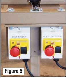
Controls switches can be mounted on the Ball Caster Tables. The reversible bracket is included with each DBS machine and can hold one or two switches.
