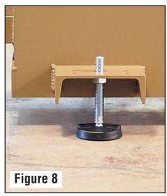
Thread the levelers into the mounting plates on the machine with the nut under the plate. After the machine is level, tighten the nuts on each leveler.
