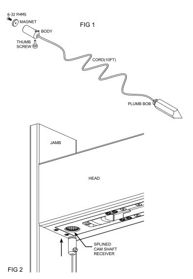
3. Adjust the head and/or sill until the plumb bob is directly centered over the gearbox. (FIG. 3)
