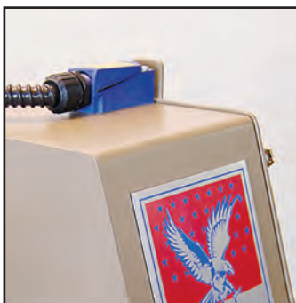
This is the Limit Switch on top of the 3300RP. Whenever the Belt Door is opened this switch will shut the power to the machine off.
