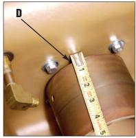
**Photo 4.** Measure Pulley to tank distance "D" before removing Lower Pulley.
