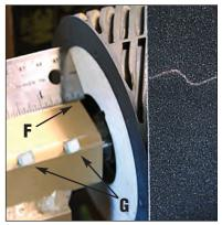
Photo 6. Measure Pulley to bracket clearance "F" before removing the Roller Platen. Loosen two Square Head screws "G" to remove the Roller Platen.
