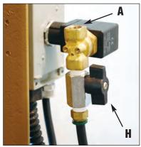
**Photo 1.** Electric Water Solenoid, Valve and Quick-Connect Fitting. Connect water supply at "A" -1/4" NPT. Water Flow Control Valve "H" can be used to regulate water spray.
