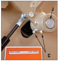
**Photo 3.** Square Head Screws "C" holding the Upper Pulley Shaft "J". Loosen these to remove the Upper Pulley Assembly.
