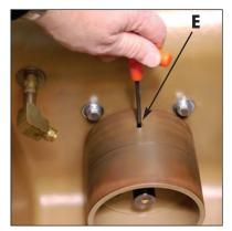
**Photo 5.** Loosen two set screws on the Lower Pulley with a 5/32" Hex/Allen wrench. Holes in the Pulley "E" line up with the two set screws.
