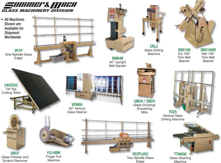
The Sommer & Maca Glass Machinery Company has built and serviced innovative, specialized machinery for the glass industry for over 80 years. Sommer & Maca machines are built to exact specifications and tested by machinery experts, then crated and shipped for use throughout the world. An extensive inventory of service parts is maintained, and trained technicians can provide installation and service assistance for the entire line.
