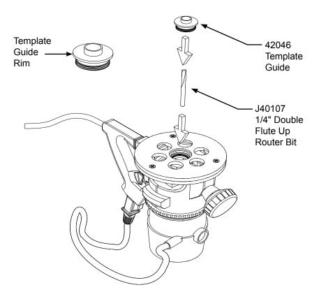
5. A 5/16" starter hole can be drilled in the center of the cut-out area in which to insert the router bit or you can plunge the router by resting the base plate edge on the work and slowly droping the spinning bit into the aluminum. Take care to hold the router firmly to prevent walking.
