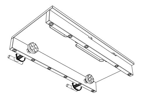
2. Insert the jamb extrusion into the jig and position it into place.
