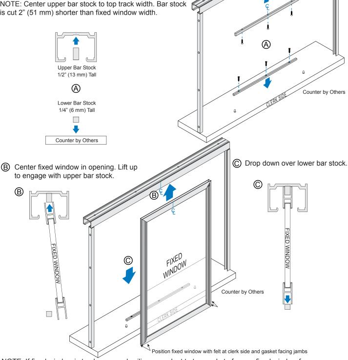
NOTE: If fixed window is too loose, apply silicone sealant to top pocket of upper fixed window frame.
