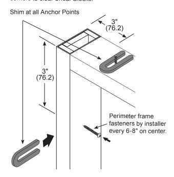
Shim and secure Door Frame to Rough Opening. NOTE: Drill holes between Door Stop Clips. Do not over tighten.
