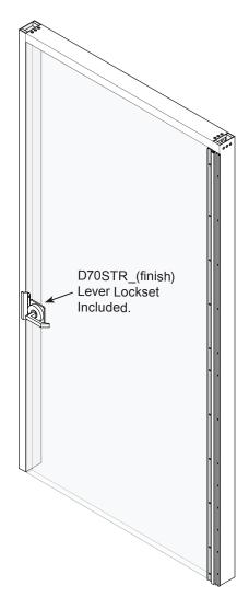
With door in place, check swing and latching. Re-adjust if necessary.
