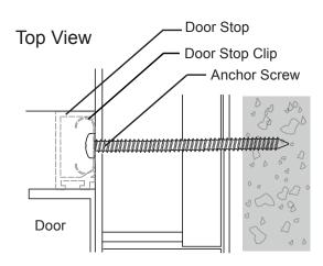
The Door and Frame are shipped separately. The Gear Hinge is attached to the Door at the factory. The Door Stops are shipped loose. This will allow the Anchor Screws to be installed around the Frame perimeter, between the Door Stop Clips, and then covered by the snap on Door Stops.
