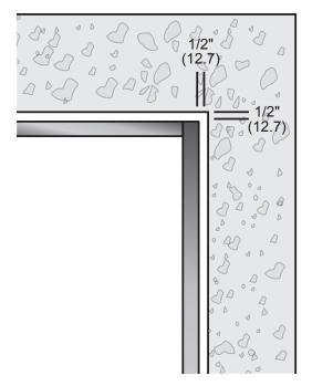
Rough Opening should be 1/2" larger than Frame at Jambs and Head. RO Width = Frame Width +1" RO Height = Fame Height +1/2"
