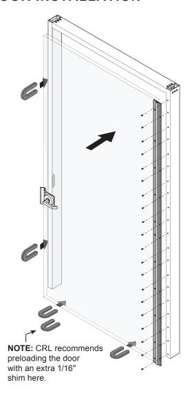
Open the Gear Hinge to 180° degrees and place the door in the frame. Center and Gap using shims. Drill holes through hinge into frame and insert twenty #12 x 3/4" undercut Phillips flat head self-drilling screws. (Supplied, see small hardware pack)
