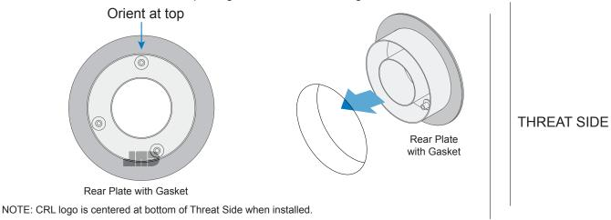
Align screw holes in parts and center in opening. Tighten screws evenly but do not overtighten.
