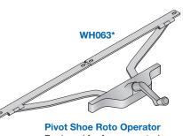
Designed for face mounted applications on single vent awning windows, this operator's unique pivot shoe design allows approximately 10" (254) of opening. Acetal pivot shoes slide smoothly in the track assuring positive operation and creating a self cleaning action.
