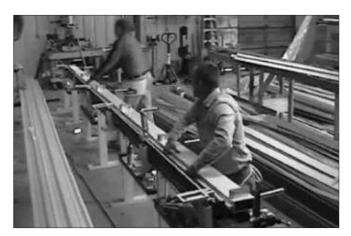
2. Release the pneumatic clamping system and flip up the jigs.
