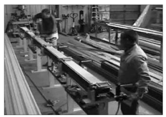
8. Release the pneumatic clamping system.
