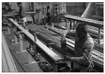
6. Flip down the jigs and begin to install Shear Blocks on the reverse side.
