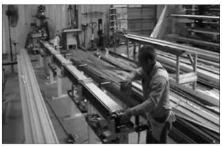
With the pneumatic clamping system on, set the jigs to their proper locations and begin fastening Shear Blocks to one side of the Curtain Wall's Vertical Mullion. Proceed down the Vertical Mullion until all Shear Blocks are installed.
