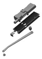
(7) - Concealed Connecting Arm Wrought metal arm connected directly to door to provide a strong, triangular positive stop at 90 degree opening and prevent stress at the header to jamb connection. Constant check control avoids abrupt rebounding of door.
