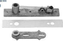
The CRL Jackson Center-Hung Pivot Set is designed to be used with standard 1-3/4" (44 mm) storefront aluminum doors weighing up to 250 pounds (113 kg). These Pivots fit top door rails with a depth of 1" (25 mm) and drops down 3/4" (19 mm) for full contact with the included Top Door Pivot Arm. Pin diameter is 1/2" (12.7 mm). These are perfect for new or retrofit applications.
