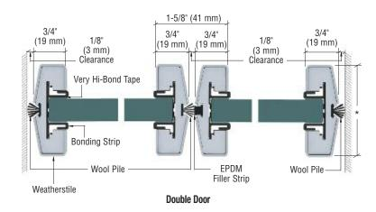
\* Overall width is 2" (51 mm) for 1/2" (12 mm) glass; 2-1/4" (57 mm) for 3/4" (19 mm) glass.
