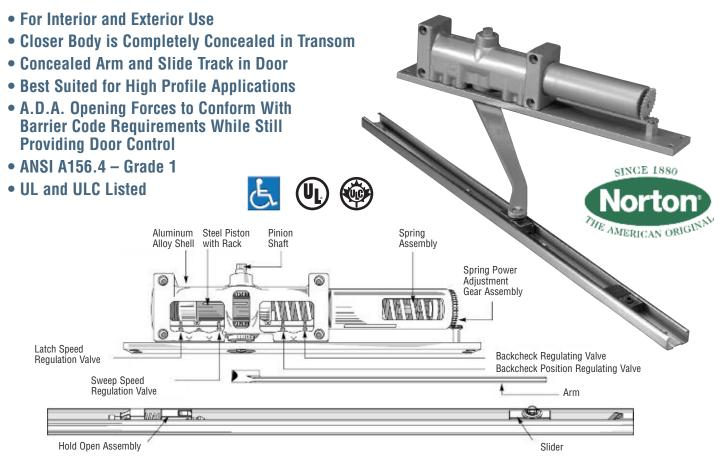
Overhead Concealed Door Closers provide an aesthetically appealing way to close a door. In situations where a closer is needed but concealment in the frame header is required or desired, the Norton® 7900 Closer is the ideal solution for door control. Once installed, only the solid one-piece arm is visible when the door is open; therefore, this unit provides a high degree of vandal resistance. When the door is closed, the closer, arm and slide track are fully concealed.
