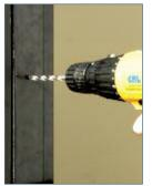
First, drill the appropriate size hole for the Rivet-Nut into your door or drill out the old, stripped thread insert.
