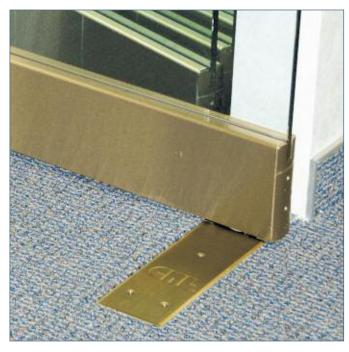
These Shallow Depth Floor Mounted Door Closers are preferred for many types of installations because they only require a shallow 1-9/16" (40 mm) cut-out in the floor. This is especially important on floors above the ground floor. The shallow cut-out leaves enough remaining floor under the Door Closer to support the door weight. The Door Closer has separate valves to control closing and latching speeds. Both 90 degree and 105 degree Hold Open and No Hold Open models are available.
