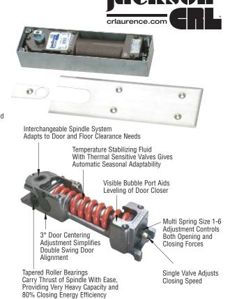
**NOTE:** This Door Closer is designed to open to a maximum of 180 degrees. An auxiliary floor or overhead stop is required to stop the door at less than 180 degrees.
