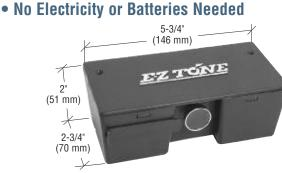
The EZ Tone can be easily installed on all types of doors and jambs. When the door is opened, a magnetic striker hits the chime bar and produces a pleasant, audible tone.
