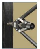
Third, compress the Rivet-Nut by using the CRL Cat. No. 34604 Heavy-Duty Thread Insert Tool
