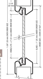
CRL's new Door Vision Lites are constructed from 20 gauge CRS bronze powder coated frames. They are designed for 1-3/4" (44 mm) thick doors in sizes from 5" x 35" (127 x 889 mm) to 24" x 60" (610 x 1524 mm). Vision Lites include mitered and welded corners, a continuous glass retainer, and countersunk mounting holes in the bevel on the non-corridor side. These Vision Lites are listed with both UL and WHI. Custom sizes and finishes are available upon request.
