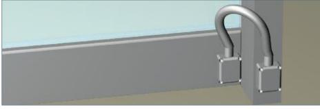
Rail Mount Detail at Sill/Jamb and Wire Loop for EG110
