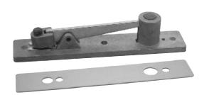
This Center-Hung Top Pivot fits top door rails with a depth of 1" (25 mm). Hardened steel pin has a diameter of 1/2" (12.7 mm), and drops down 3/4" (19 mm) for full contact with Top Door Pivot Arm.
