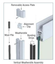
NOTE: CRL Vertical Weatherstiles are intended only for use on newly fabricated doors being installed into a new or existing opening. They cannot be
