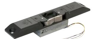
SPECIFICATIONS: Input: Field Select 12V AC/DC 24V AC/DC Contact Technical Sales for 16V AC/DC Current Draw: .44A @ 12V DC .16A @ 12V AC .23A @ 24V DC .08A @ 24V AC Case: 1" x 3-3/8" x 1-1/16" deep Dimensions: (25 mm x 86 mm x 27 mm) Strike Opening: 5/8" x 1-7/16" x 9/16" (16 mm x 37 mm x 14 mm) Shipped as Fail-Secure Lock: Requires Power to Unlock. Field Convertible to Fail-Safe Mode.
