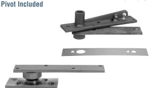
This Rixson<sup>®</sup> Center-Hung Pivot Set features a 500 pound (227 kg) weight capacity, and can be used on doors up to 44" x 102" (1118 x 2591 mm). Double-acting non-handed Bottom Pivot mounts directly to floor. Sealed bearings for protection against the weather.
