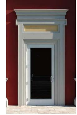
The BAL-350 is designed to accommodate 9/16" impact resistant glass. Each door is factory glazed using square glass stops with our wet/dry glazing method using a combination of Tremco EPDM spacer and wedge gasket along with DOW 995 for the internal silicone seal. Further increasing our impact resistance, Delta Doors equips each BAL-350 door with non-removable exterior glass stops.
